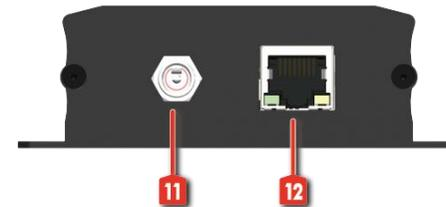
11. **Latch-locking power jack:** Connect to 12V DC power supply
